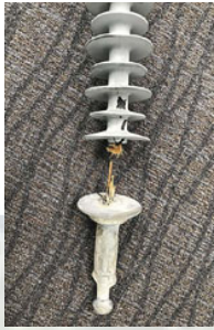
Picture Left: Insulator Failure due to Corona
