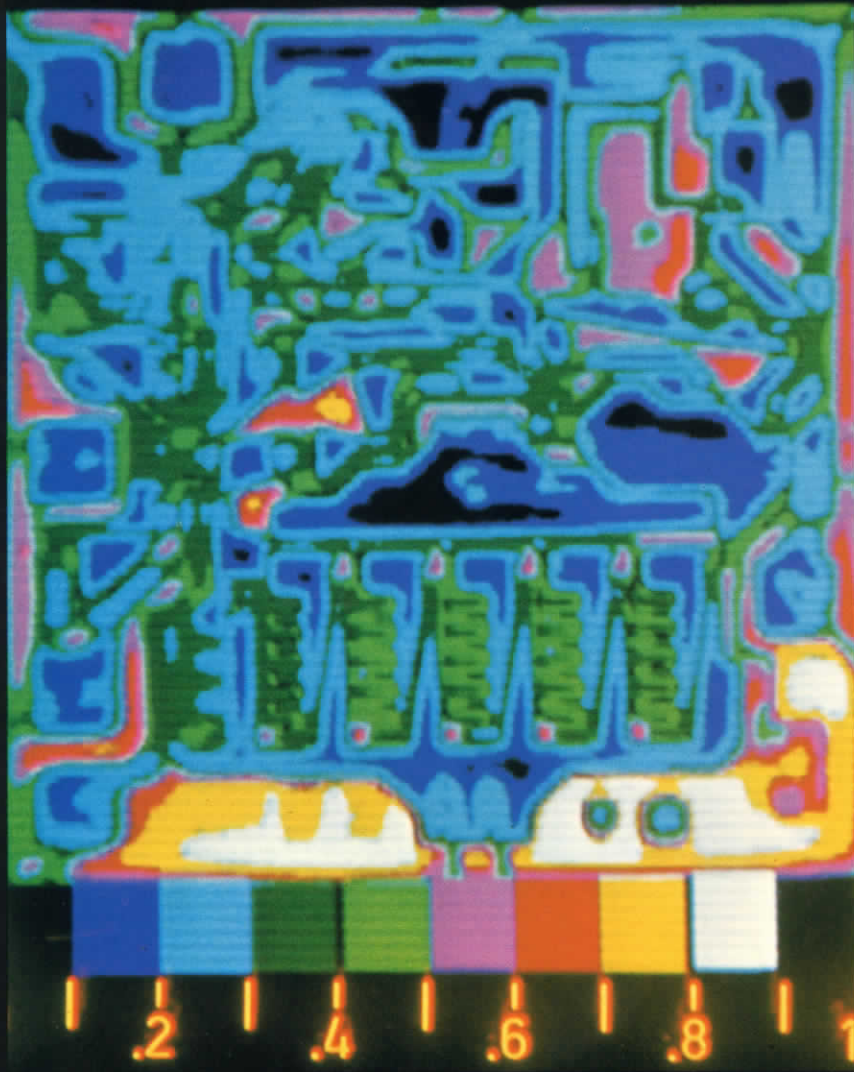
Thermogram of a regulator circuit with associated resistors, transistors, etc. The energized circuit, potential failure areas appear as very hot parts, shown in white, yellow, and red. Each color represents a temperature differential of 5 C.
