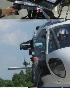
280 nanometer band for interference free reception of the Corona Emission UV radiation
