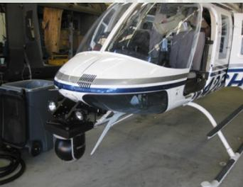
Picture to the left shows an EIR/SWE 300 installed on a Bell LongRanger helicopter with a nose mount.
