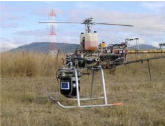
**The easy adaptability and ruggedness of the EIR/SweSystem Gimbal camera packages have made them popular for many special applications. The picture to the left shows an Unmanned Air Vehicle using the SWE300 gimbal for inspection of electric power lines!**
