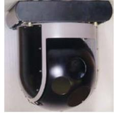
**Instead of using an Infrared camera with complex and expensive optical zoom, we are using two cameras in the gimbal with different lenses: 25mm (8° x 6° FOV) and 100 mm (34° x 25° FOV). These cameras now have 640x480 pixel resolution and high sensitivity. This means that you can display both images at the same time or have them switched from wide to telephoto.**
