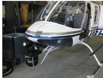
Other IR camera-lens configurations are available. Two small Tau cameras with 25mm and 100mm lenses plus Sony FCB H11 will fit nicely.
