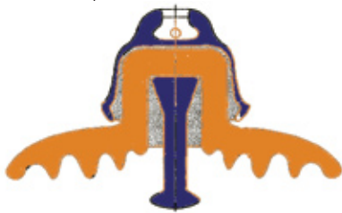
Figure 1 Section view of a porcelain insulator
