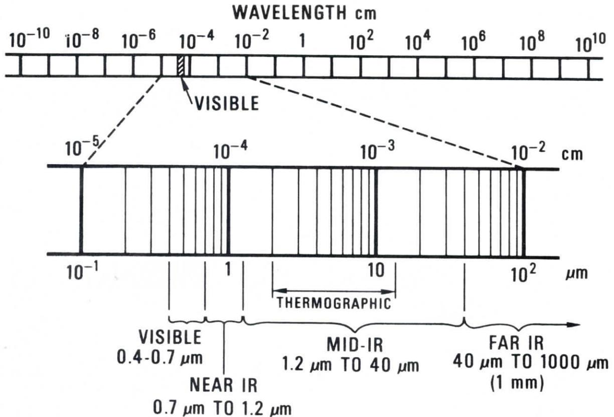
**FIGURE 1** The Electromagnetic Spectrum from  $10^{-10}$  cm to  $10^{10}$  cm wavelength, with detail of visible and infrared (IR) wavelengths.
