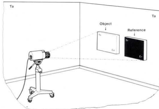
FIGURE 3 Principle of absolute temperature measurements
