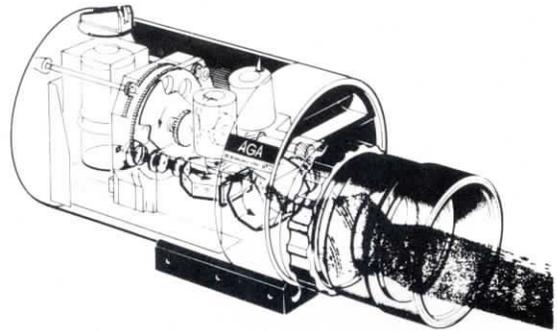
**FIGURE 4** Phantom view of thermal imaging camera. The dark band represents path of energy in the system. The first rotating prism generates vertical scan, the second prism generates horizontal scan. The detector is at the bottom of the liquid nitrogen container at the rear of the camera. Aperture disks and chopper are in front of the detector. (Courtesy of AGA Infrared Systems, AB.)
