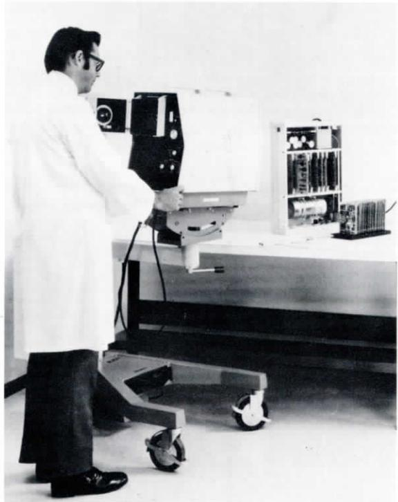
**FIGURE 9** The Spectrotherm Model 800 thermal imaging system. The video display is integral with the camera housing. (Courtesy of the Spectrotherm Company.)
