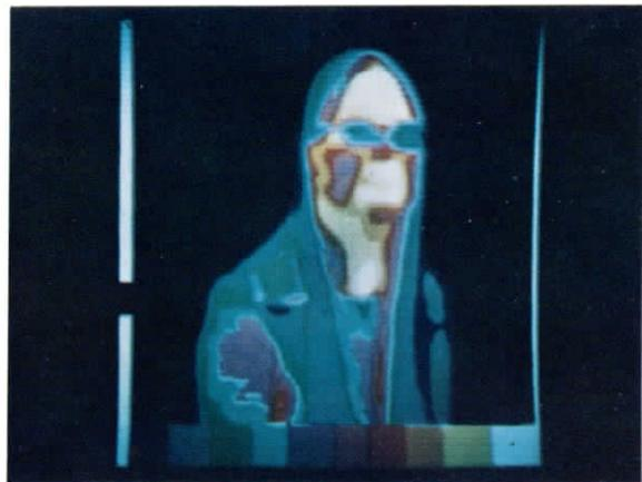
**FIGURE 6** Thermograph of Figure 5, made on color monitor designed to display isotherms, or areas where radiation is of like intensity. The colors are arbitrary and chosen to separate total range of energy into 10 discrete steps. Blues and greens indicate lower range, reds and yellows the higher range. The isotherm presentation helps in assigning temperature to various parts of an image.
