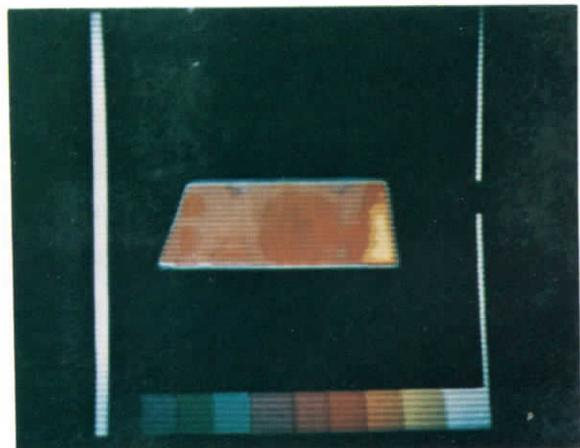
FIGURE 10 Thermograph of plate slab just after the first mill stand, showing temperature gradients.
