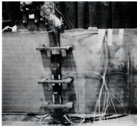
**FIGURE 12** Photograph of electroslag welding experiment. The vertical channel will contain the weld area. Wire are to thermocouples.
