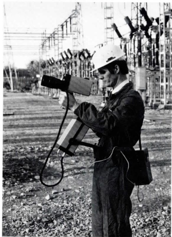
**FIGURE 1** Portable AGA Thermovision Model 750
