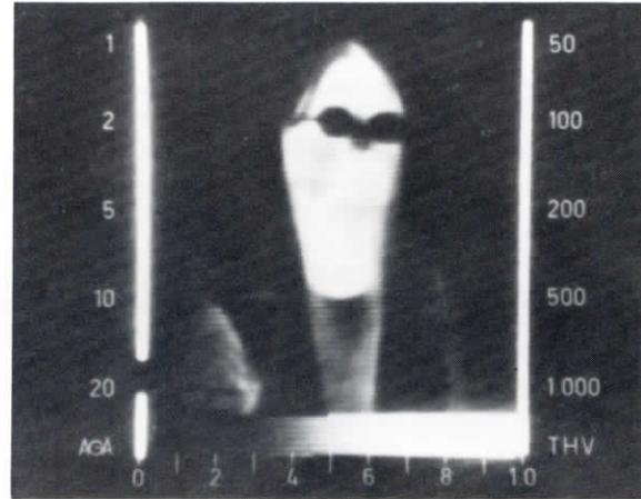
**FIGURE 5** Photograph and thermograph compared. Skin area radiates the most energy and appears lightest. Hair radiates little energy because it is cool and appears dark. Lapels on dress are darker than dress because they are cooler due to added layers of cloth. Glasses appear dark because optical glass doesn't transmit infrared energy at the wavelengths used.
