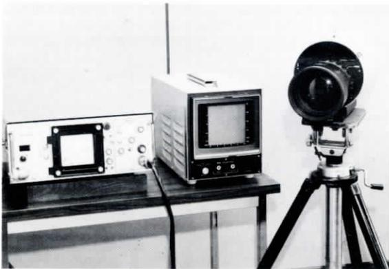
**FIGURE 7** The camera, the camera control and video display unit, and the color monitor of the AGA Infrared Systems AB, Thermovision®, Model 680.
