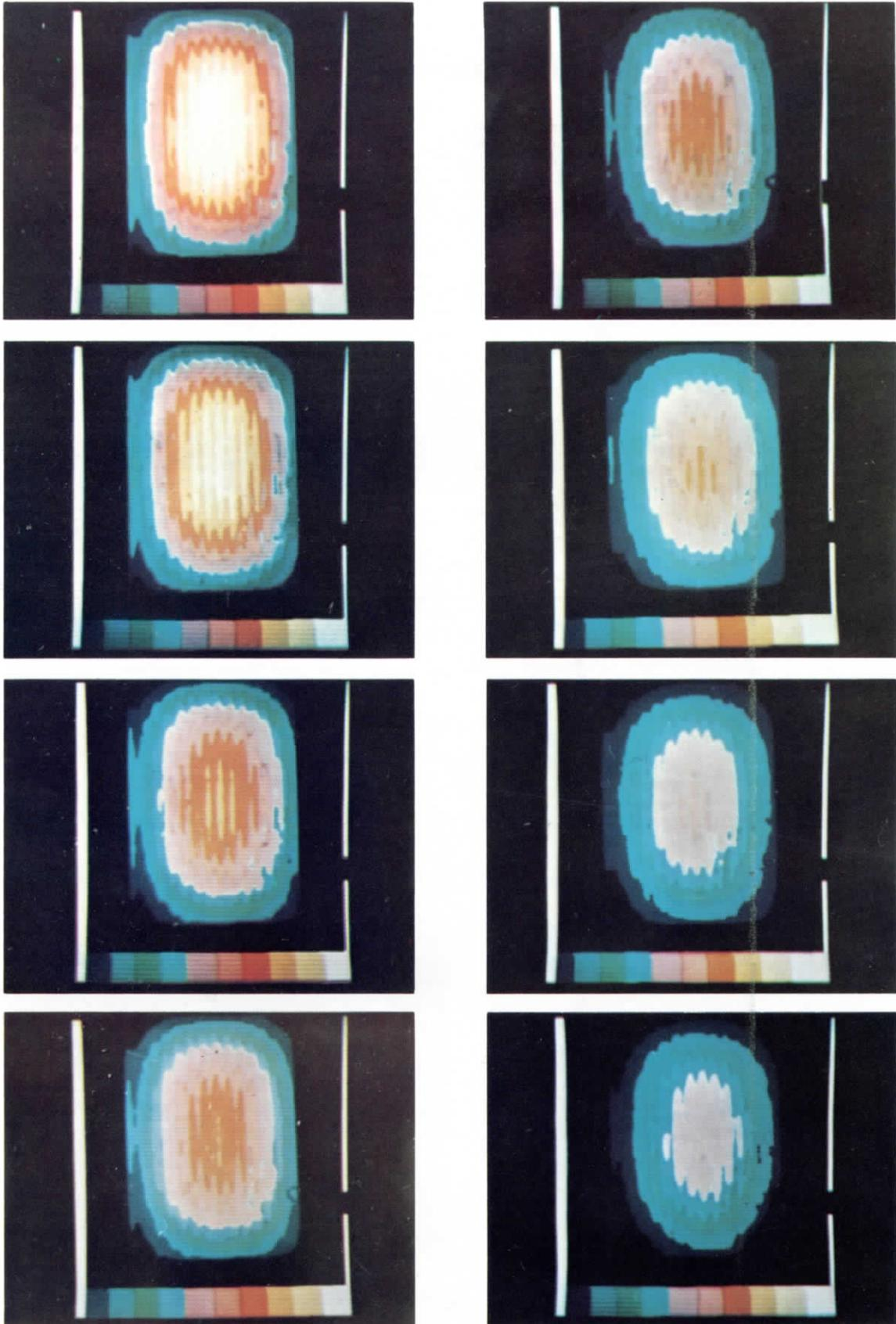
FIGURE 11 This series of themographs show the progressive thermal patterns on the surface of a cooling ingot.
