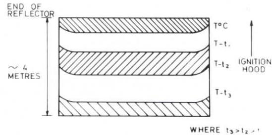
FIGURE 2 GRAPH SHOWING EXPECTED ISOTHERMS OF AN IDEAL SINTER STRAND
