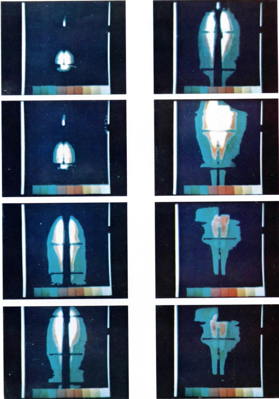
**FIGURE 13** Series of thermographs showing progress of thermal pattern spreading away from the electroslag weld as the welding progresses.
